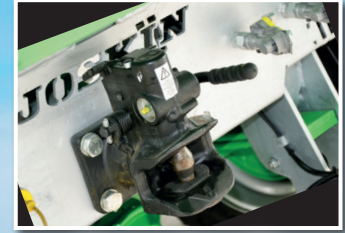
Rear automatic yoke with complete equipment
